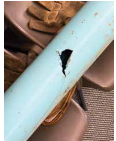
The photos pictured above left show the device that was used to damage the PVC water line (pictured) causing a 350,000 gallon leak.
