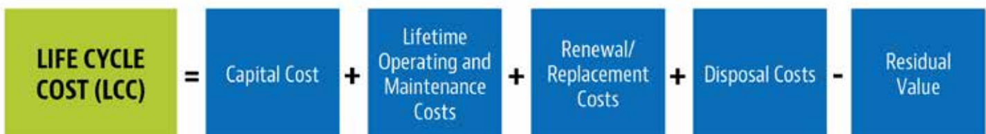
Figure 2: Life Cycle Cost Analysis Equation
