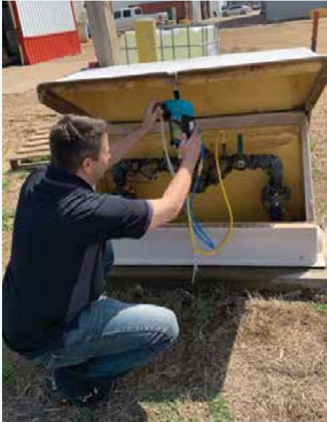
Steve Attema finishes up a successful test of a "RP" Backflow assembly. Steve performed two tests, the first at a dairy near Parker, SD and the second at a Coop fertilizer site near Marion, SD. SDARWS did the testing at the request of TM Water User District.
