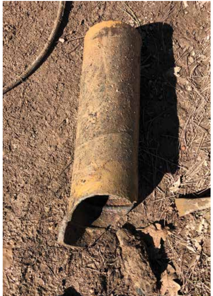
A valve riser that was set too high and hit by a snowplow.
