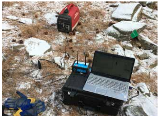
Correlation equipment being powered by a generator to test the water main
