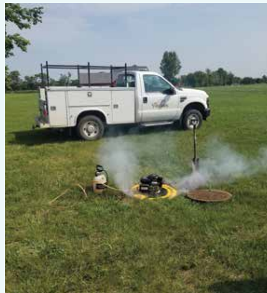
SDARWS Training and Technical Assistance Specialist was recently in Parkston assisting with smoke testing.
