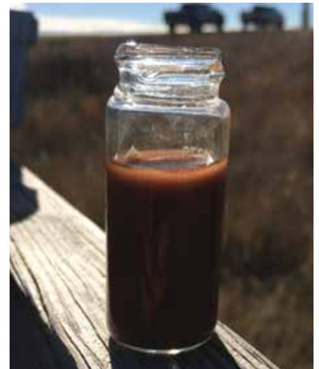
300 mg/l sample taken from water main
