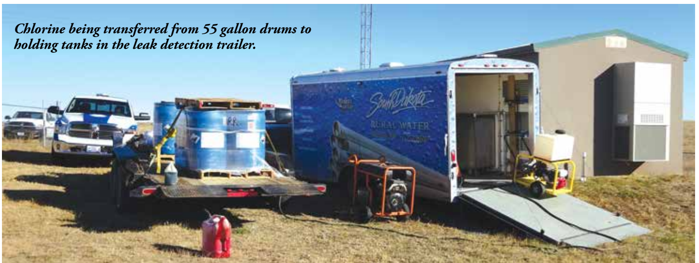
Leak detection trailer hooked up to pump station and hose running to the chlorine injection point.
